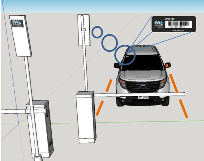
The sticker ID received by the transmitting antenna in the range of about 3 to 7 meters from the antenna base and depends on the environment. Height of the antenna should be about 1.5 to 2.5 from it's base.
