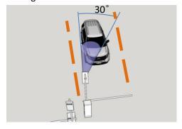
The sticker ID can be received by RFID device up to 7 meters (23 feet) from the antenna base and depends on the environment.
