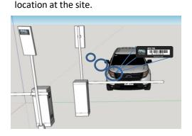
The antenna is transmitting via cone of approximately 30 degrees.
